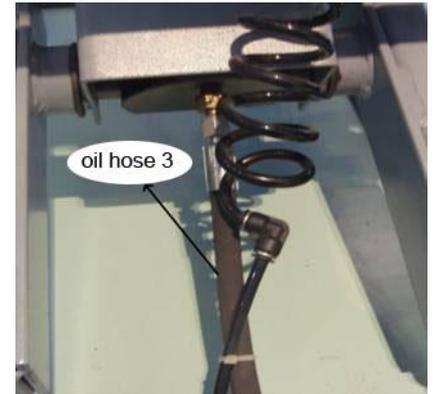
**Step 3:** Connect the pneumatic release system by referring the following pictures.
